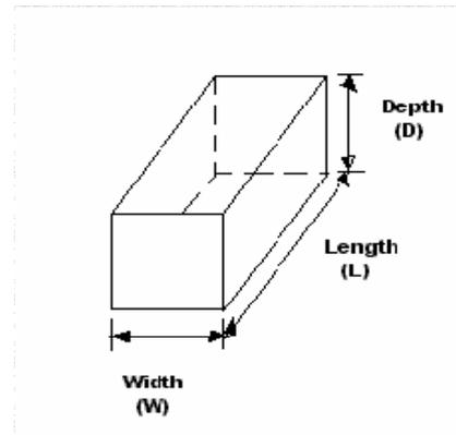
Other forest products such as lumber, shingles, plywood, staves assume the shape of a cube. The volume of a cube is calculated using the formula  $W \times D \times H = V$ , where  $W$  is the width,  $D$  is the depth or thickness,  $H$  is the height or length, and  $V$  is the volume.
